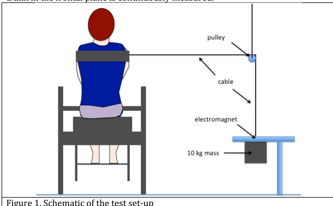
Figure 1. Schematic of the test set-up
